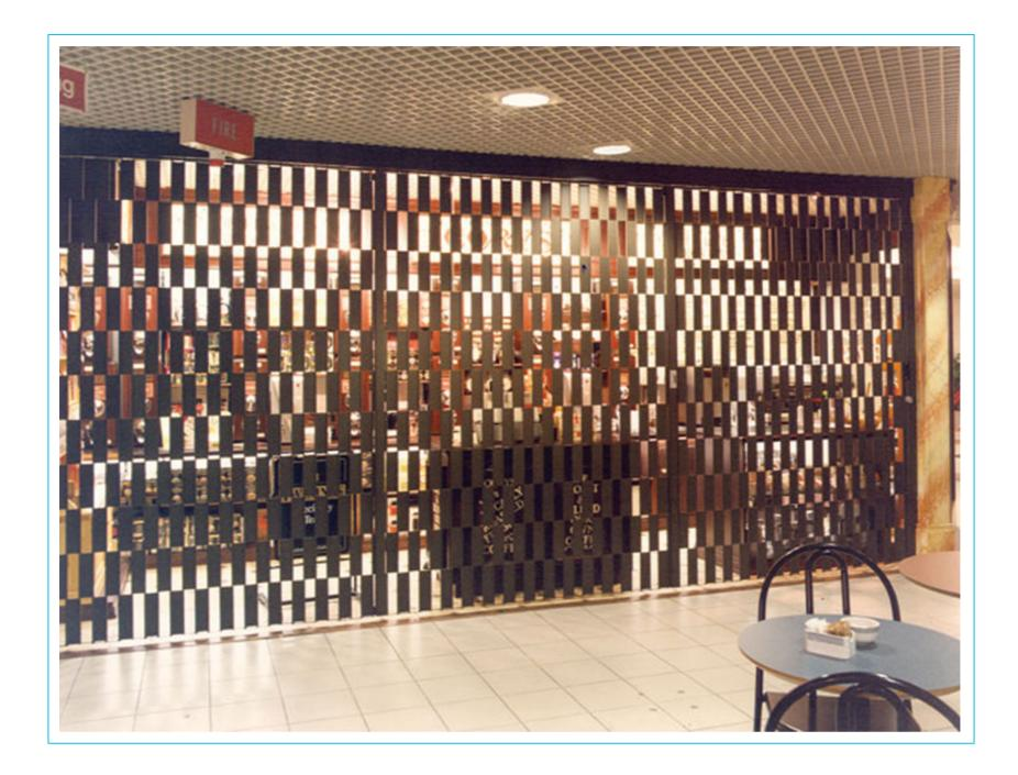
A manually operated folding sliding aluminium grille that provides a good level of security. Gaps within the checker plate design allow for through vision. A selection of finishes are available and Adams Rite mortice lock fitted as standard. Suitable for curved apertures. No maximum span. Recommended maximum height up to 4,500mm.
